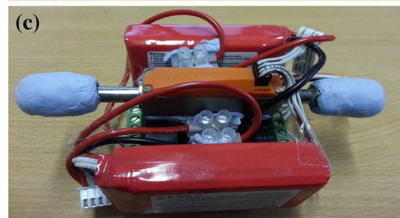
Fig. 9 CAD Design and Implemented Capsobot. a 3D CAD design of the Capsobot (without Capsobot-shell). b Implemented Capsobot: With Capsobot-shell. c Implemented Capsobot: Without Capsobot-shell
